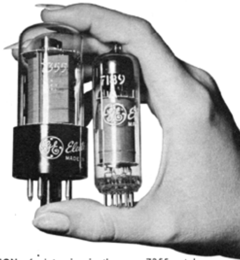
COMPARISON of plate size in the new 7355 octal beam pentode (left), and the 7189A miniature beam pentode (right). The tubes have design maximum plate dissipation ratings of 18 and 13.2 watts, respectively.
